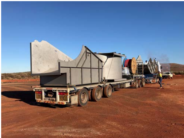
Figure 1. Large custom mining fans are transported in pieces and assembled at the site.
