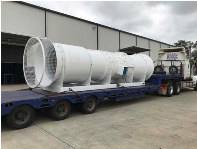
Figure 4. Twin axial booster fans – part of overall ventilation demand upgrade (132 - 1400 kW).
