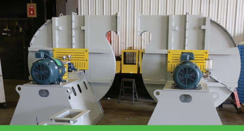
construction, split housings, independent pedestals, liners, elevated temperatures, alloy construction, gas tight construction, etc.
