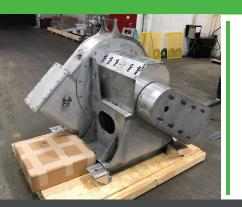
The New York Blower Company manufactures fans for sanitary applications, such as dairy processing, food and beverage processing, and pharmaceutical production. These fans must adhere to stricter regulations, and are constructed based on ease of maintenance and accessibility, minimizing potential complications, and performing up to expectations.
