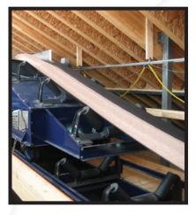
Tripper cars are instrumental to grain storage. Tripper cars provide unique opportunities for hazard monitoring as the movement makes Class II Div. 1 monitoring difficult. HazardPRO wireless sensors can be mounted directly to the tripper car, providing monitoring for speed, temperature and alignment. Wireless hazard monitoring provides a solution to the most difficult equipment to be monitored in your facility.
