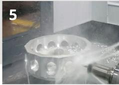
The pictures show the process of the EC1600 machine cutting blade pickets of a 24" .60 ratio Variable Pitch Vaneaxial wheel hub from steps 1 through 5.
